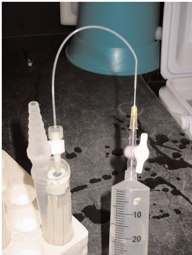
Fig. 1. Injection of the headspace gas into the Exetainer vial. The needle extender allows the sample syringe to be maintained with the headspace at the top while injecting the gas into the Exetainer, the septum of which remains submerged under a few millimeters of water to ensure against air contamination. The plastic tube fitting jams the Exetainer in place so it does not float out of its water bath.
