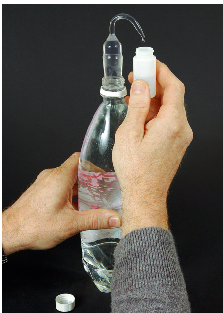
Fig. 1. Photo of the glass nozzle fitted to the PET bottle as used when displacing mineral oil to the scintillation vial.
