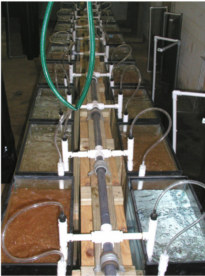
Figure 2. Photograph of sediment suspension apparatus in use.
