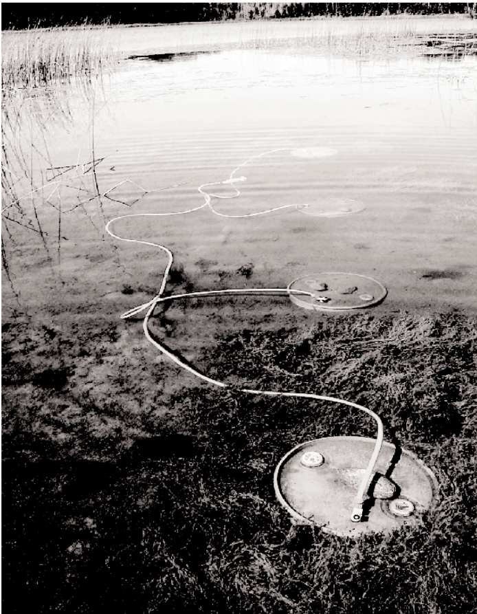
Fig. 3. Ganged seepage cylinders in Shingobee Lake, MN.
