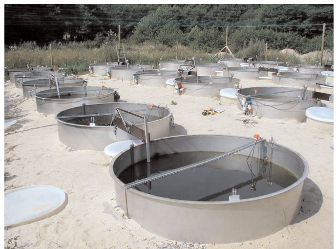
Fig. 2. Mesocosms to experimentally study how increased temperatures will affect shallow lake systems.
