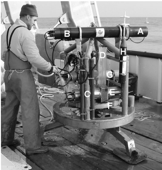
Fig. 4. INSSECT with instrumentation mounted. (A) Digital floc camera; (B) OBS mounted on rear end of DVC; (C) batteries for Digital video camera; (D) settling column; (E) digital video camera; (F) skirt (old version of sediment trap system); (G) controller for DFC and OBS; (H) MAVS current meter.
