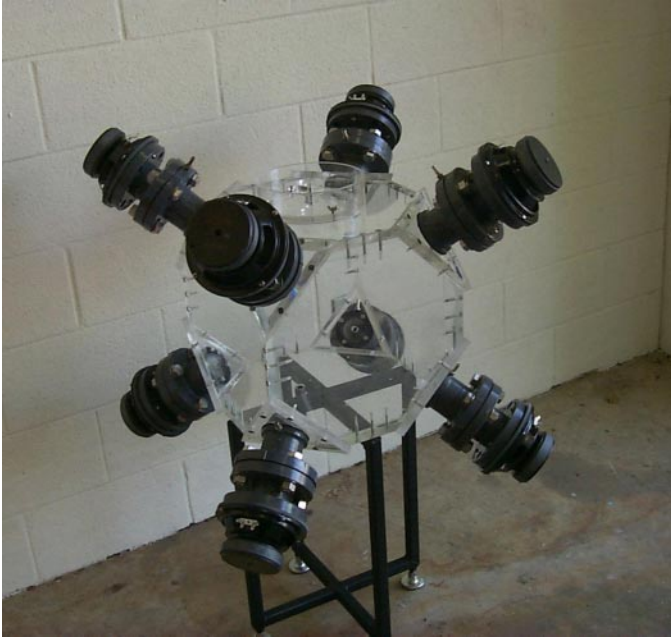
Fig. 2. Photograph of the turbulence chamber and actuators
