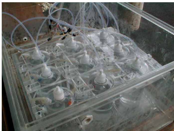
Fig. 3. Photograph of the chemostat bottles in the holder rack inside the incubator, showing inflow tubing entering through the top of the bottles and outflows at the shoulders of the bottles.
