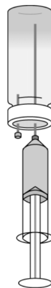
Fig. 1. Dilution of samples suspected of high N 2 concentration; 25% to 50% of the water in a vial is replaced by warm water of known gas concentration.
