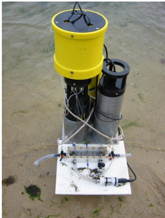
Fig. 2. The automated seepage meter showing all major components of the system except for the seepage housing.
