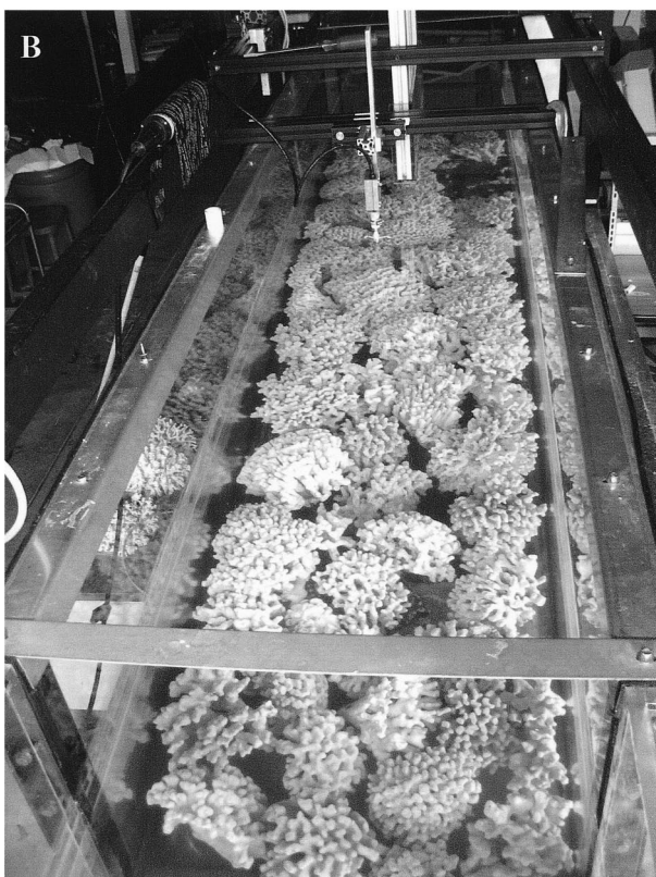
Fig. 1. (A) Schematic diagram of laboratory flume setup. (B) Photo of flume with ADV setup visible.
